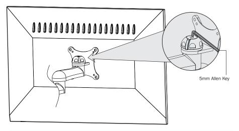
Tighten the adjustment screw by using Allen Key provided to fix the tilting angle
